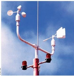
FIGURE 9.19 A wind vane and a cup anemometer. These instruments are part of the ASOS system. (For a complete picture of the system, see Fig. 3.30, p. 83.)
